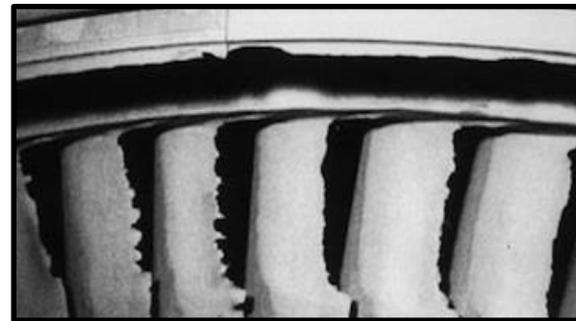
*Eroded steam turbine blades
