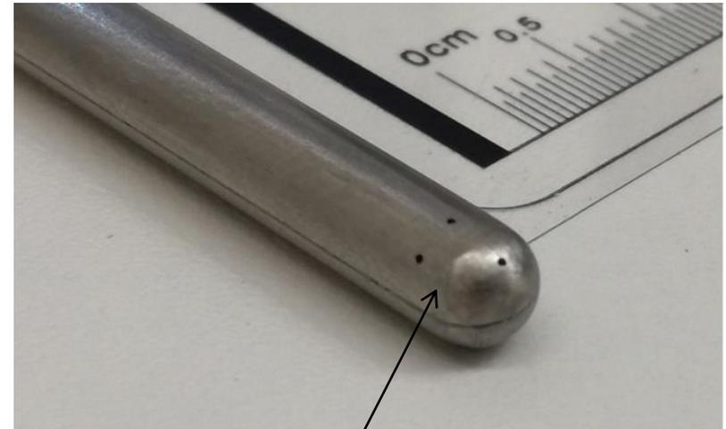
4-sensors installed in tip of  $\varnothing$  5mm
