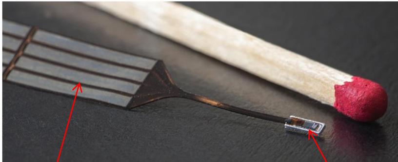
Electrical leads (75 $\mu$ m Flexible printed circuit) Bonded sensor into container (RTV coated or with «pepper pot» screen)
